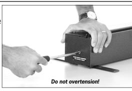
If adjustment is needed, hold the cassette firmly in place then depress and turn the adjusting screw clockwise to increase the tension (the tension mechanism adjusts in halfturn increments). Slowly release pressure on the screw turning slightly counter-clockwise and allow it to again lock in place. If tension has been lost completely, we recommend 20-25 full clockwise turns.
